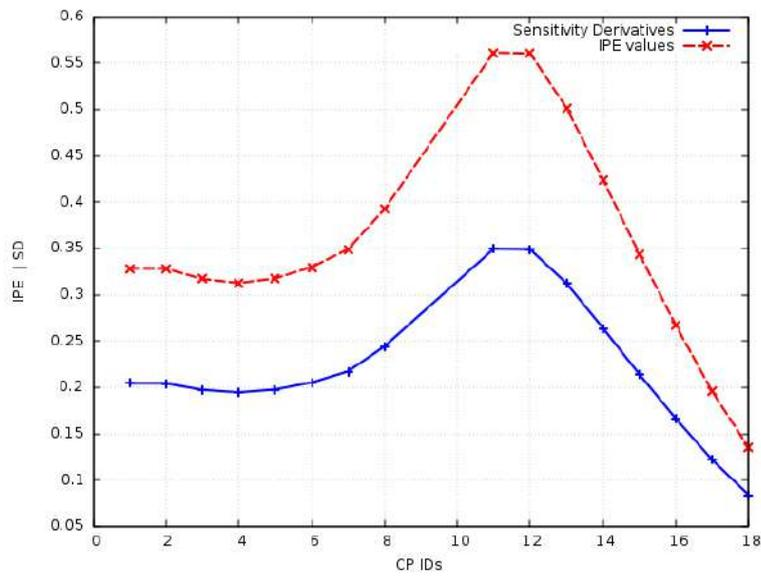
**Figure 4.10:** Study 4: Comparison of the IPE values of  $y$  coordinates of CPs for Case 5 to the absolute of the corresponding sensitivity derivatives.
