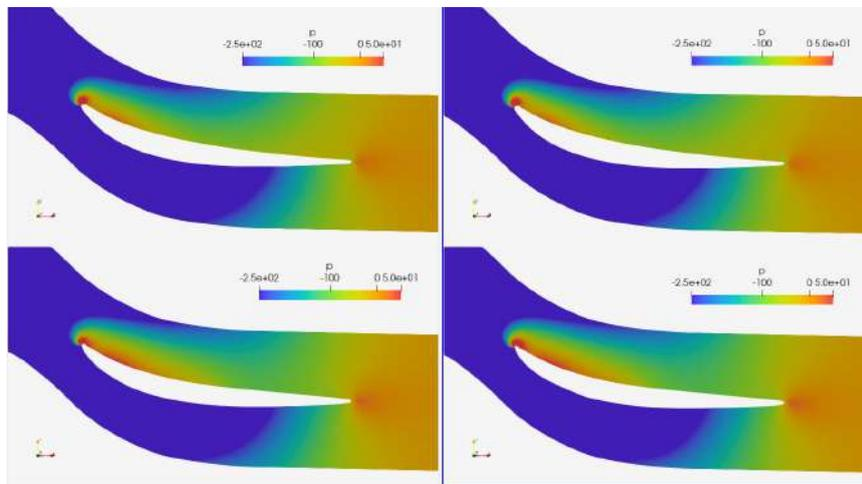
**Figure 5.22:** *Compressor cascade Optimization: Pressure fields of Cases 1(left) and 2(right).*
