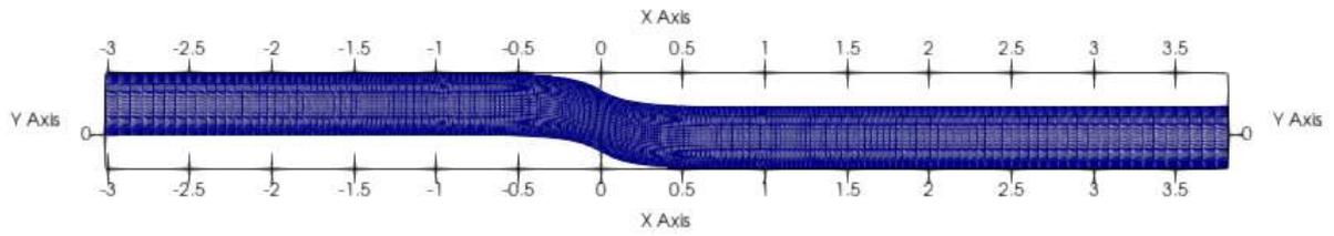
**Figure B.6:** *S-bend duct: Grid of the reference duct.*
