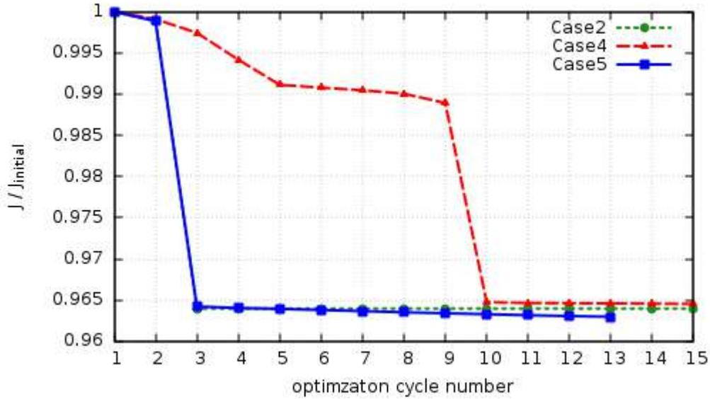
**Figure 5.10:** *Isolated airfoil optimization: Comparison of objective function values of Cases 2, and Cases 4(x coordinates) & 5 (y coordinates).*
