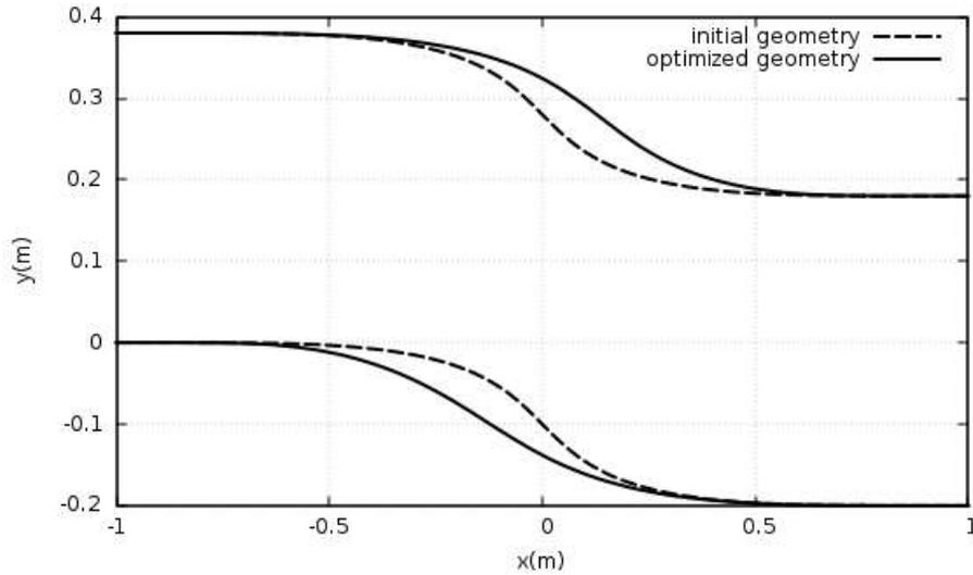
**Figure 5.16:** *S-bend duct optimization: Comparison of the optimized and initial geometry of Case 5.*
