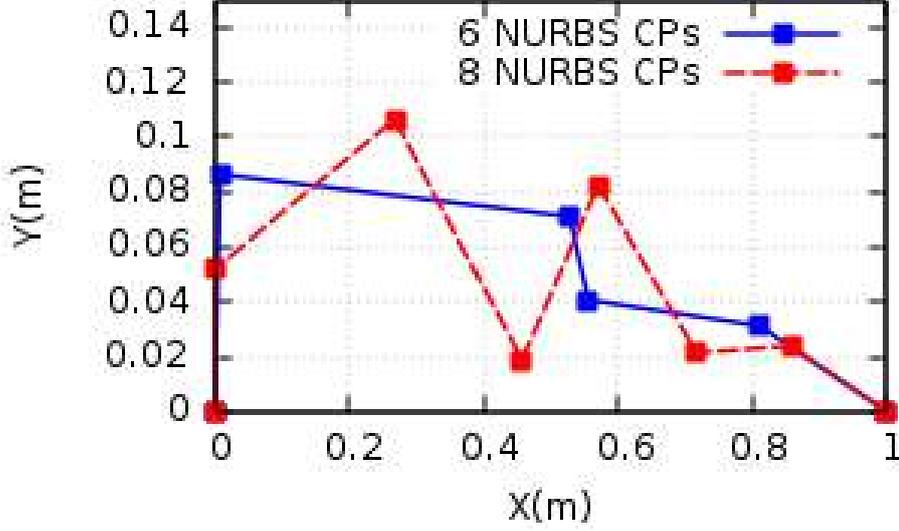
**Figure A.3:** CPs distribution of the two NURBS parameterizations using 6CPs and 8CPs.
