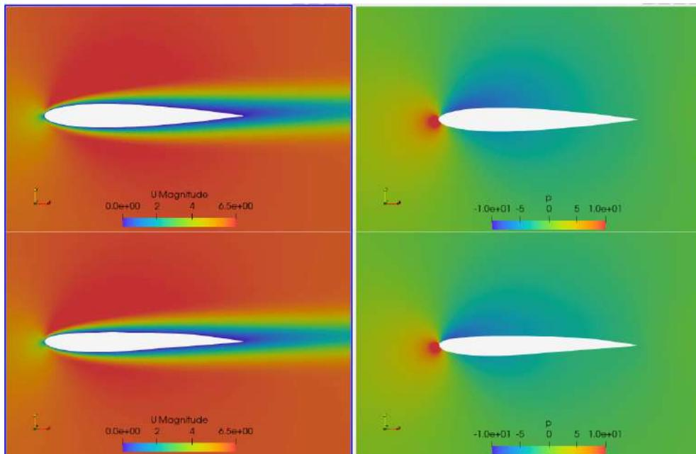
**Figure 5.4:** *Isolated airfoil optimization: Flow fields around Case 1 initial(top) and final(bottom) geometry.*
