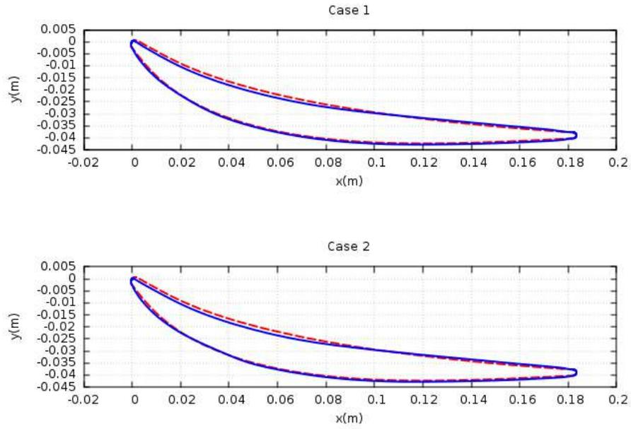
**Figure 5.21:** *Compressor cascade Optimization: Comparison of the optimized and the initial shape of each blade airfoil.*
