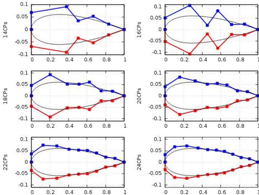
**Figure 4.3:** *Parameterizations of Study 2 using the best fit for each case's parameterization. The horizontal axis of each plot refers to the  $x$  direction whereas the vertical to  $y$  direction. All dimensions are scaled with the chord-length.*
