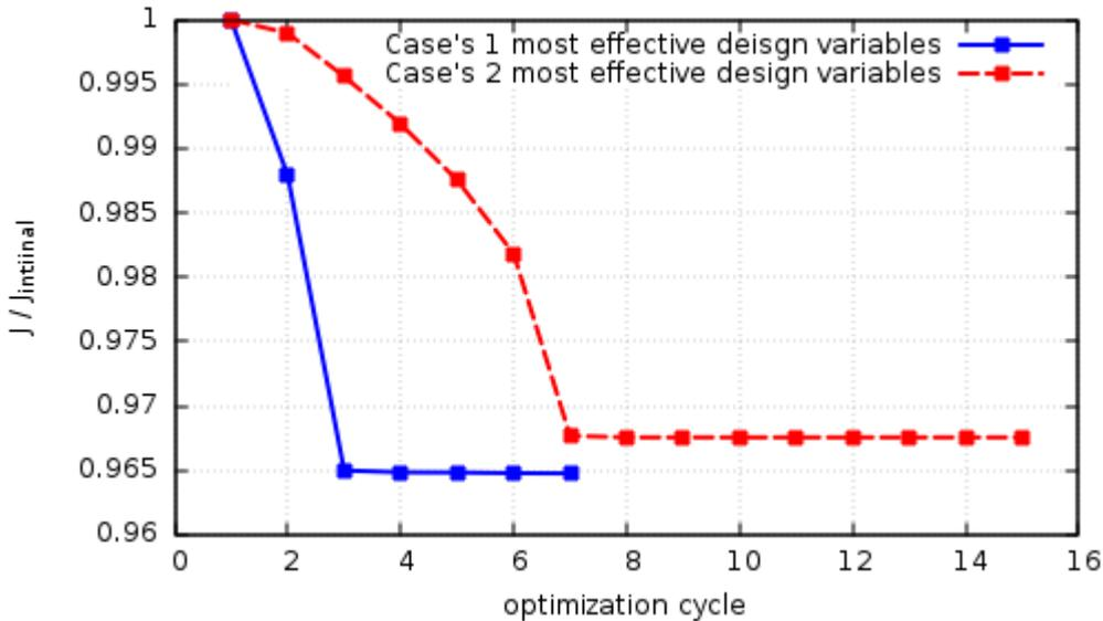
**Figure 5.8:** *Isolated airfoil optimization: Objective function values during the optimization of the Case 1 & 2 airfoils using only the 5 most effective design variables.*
