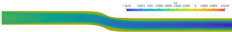
**Figure B.11:** *S-bend duct: Adjoint pressure field of the reference duct.*
