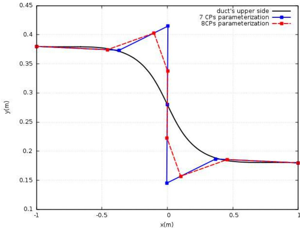
**Figure A.5:** *Enrichment of the parameterization for the S-bend's upper side.*
