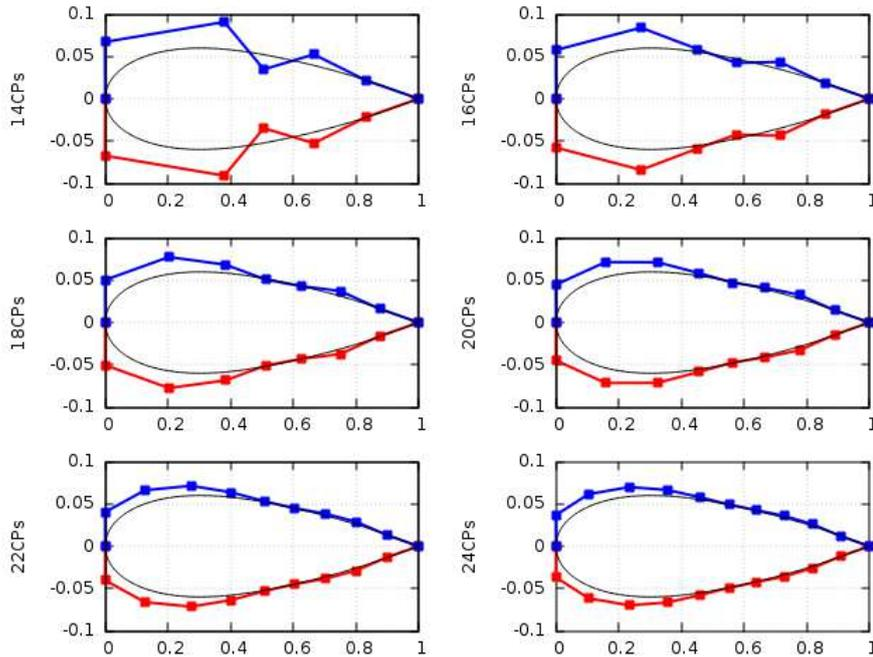
**Figure 4.2:** *Parameterizations of Study 1 using enrichment. The horizontal axis of each plot refers to the  $x$  direction whereas the vertical to  $y$  direction. All dimensions are scaled with the chord-length.*
