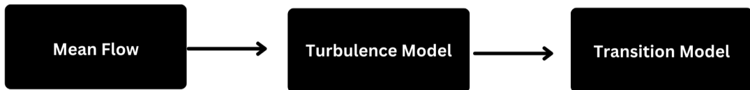
Figure 3.1: Solution of the Primal equations in every iteration. The 5 Mean Flow equations are solved producing 5 flow quantities. Next, after Spalart-Allmaras is solved for \rho \tilde{\nu} , the new value for \mu_t is obtained. Last, the two equations of \gamma - \tilde{Re}_{\theta} are solved for \rho \gamma and \rho \tilde{Re}_{\theta} .
