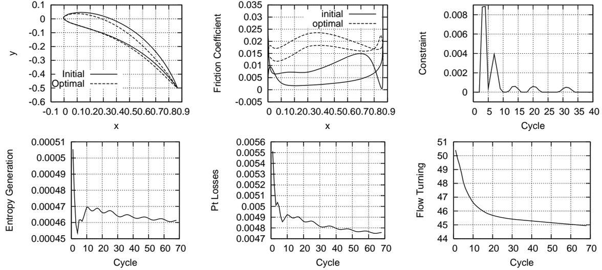
Figure 14: Losses minimization in the turbine cascade, turbulent flow. Same as in fig. 11.
