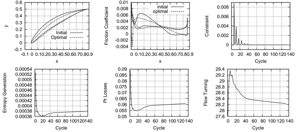
Figure 12: Losses minimization in the compressor cascade, turbulent flow. Same as in fig. 11.
