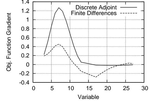
Figure 6: Losses minimization in the compressor cascade, turbulent flow: Comparison of the objective function gradient components computed using the discrete adjoint method and finite-differences.
