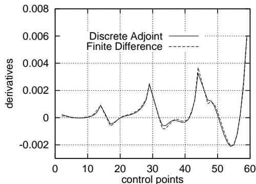
Figure 3: Inverse design of the turbine cascade, inviscid flow, unstructured grid: Objective function gradient computed using the discrete adjoint method and finite-differences.
