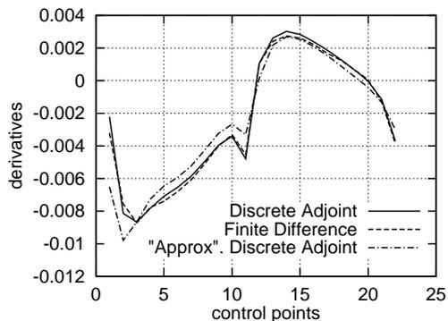
Figure 2: Inverse design of the compressor cascade, inviscid flow, unstructured grid: Objective function gradient computed using the exact (second-order accurate) discrete adjoint method, the “approximate” discrete adjoint method (second-order accuracy in the direct solver, first-order in the adjoint equations) and finite-differences.
