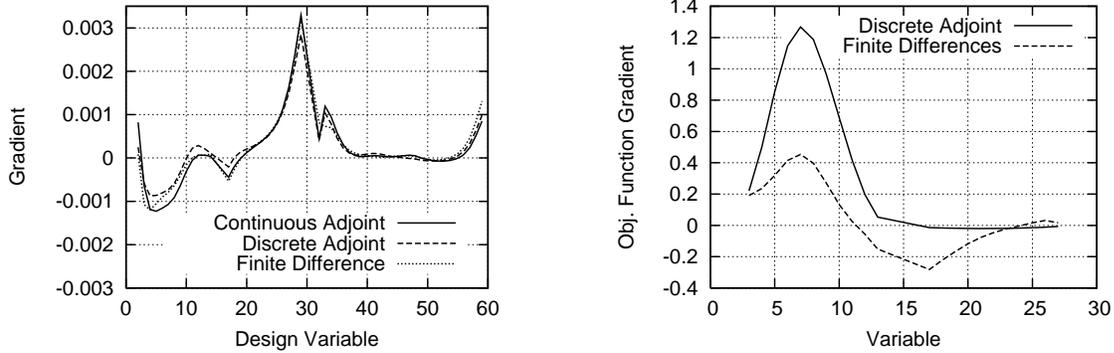
Figure 5: Inverse design of the turbine cascade, laminar flow: Objective function gradient components computed using the discrete adjoint method and finite-differences.
