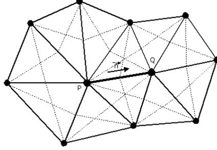
Figure 1: The flux crossing the finite-volume boundary part associated with edge PQ depends on the flow variables at node P, its neighboring nodes (including Q) as well as the neighbors of Q.
