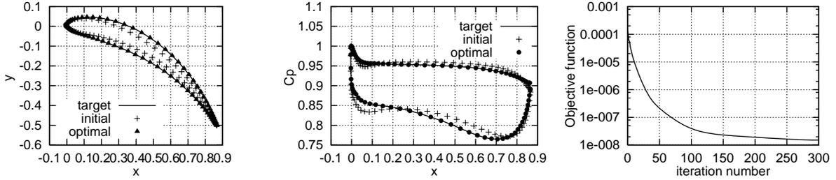
Figure 7: Inverse design of the turbine cascade, inviscid flow, unstructured grid. Left: reference, initial and optimal cascade shape, Middle: target, initial and optimal pressure distribution, Right: Convergence history.
