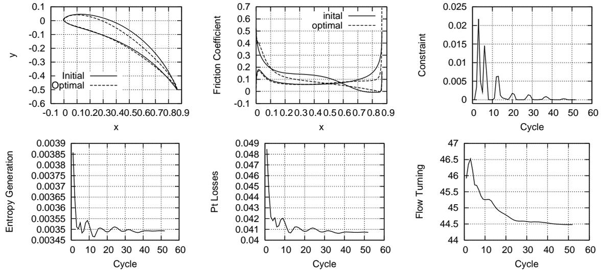
Figure 13: Losses minimization in the turbine cascade, laminar flow. Same as in fig. 11.
