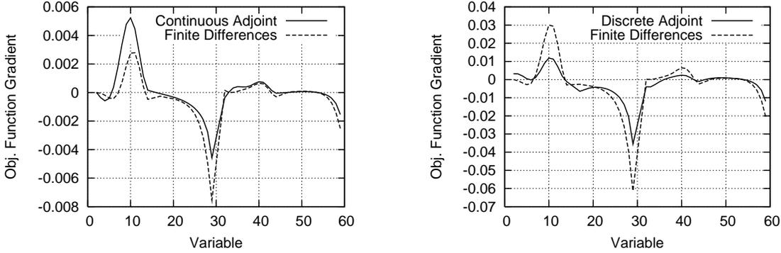
Figure 4: Losses minimization in the turbine cascade, laminar flow: Objective function gradient computed using the continuous adjoint method (left), the discrete adjoint method (right) and finite-differences.
