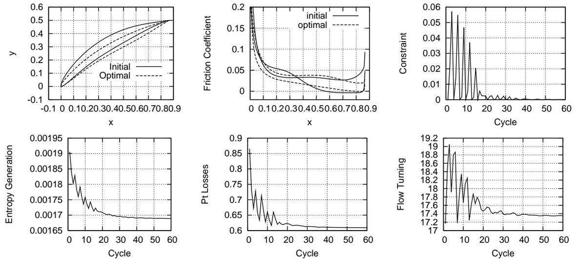
Figure 11: Losses minimization in the compressor cascade, laminar flow. Top Left: initial and optimal cascade shapes, Top Middle: initial and optimal friction coefficient distribution, Top Right: thickness deviations. Bottom from left to right : Entropy generation, total pressure losses and flow turning.
