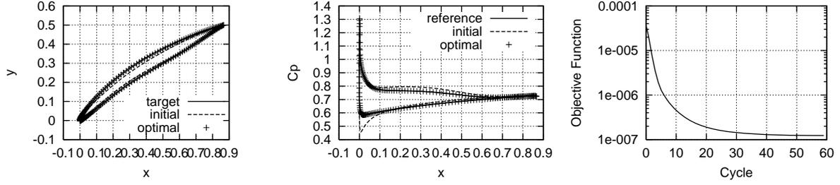
Figure 10: Inverse design of the compressor cascade, laminar flow. Same as fig. 7.
