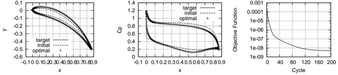
Figure 9: Inverse design of the turbine cascade, laminar flow. Same as fig. 7.
