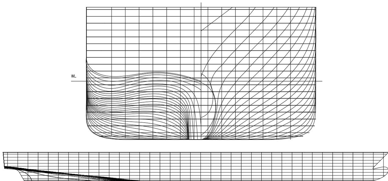
**Figure 2: Body Plan and Profile of the parent of fast displacement hull form**
