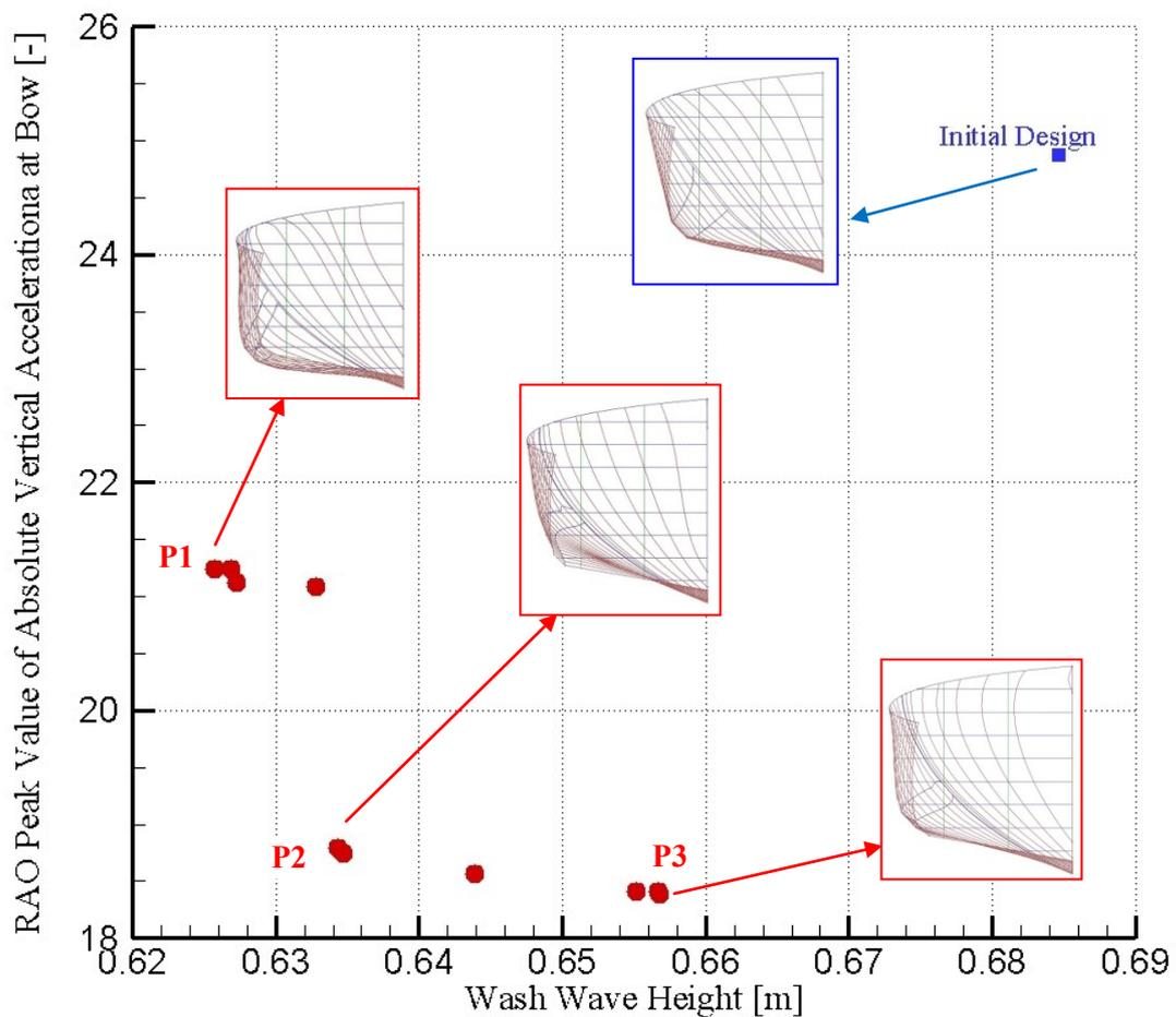
**Figure 7: Double-chine hull form design. Front of non-dominated solutions obtained using the DMAEA.**
