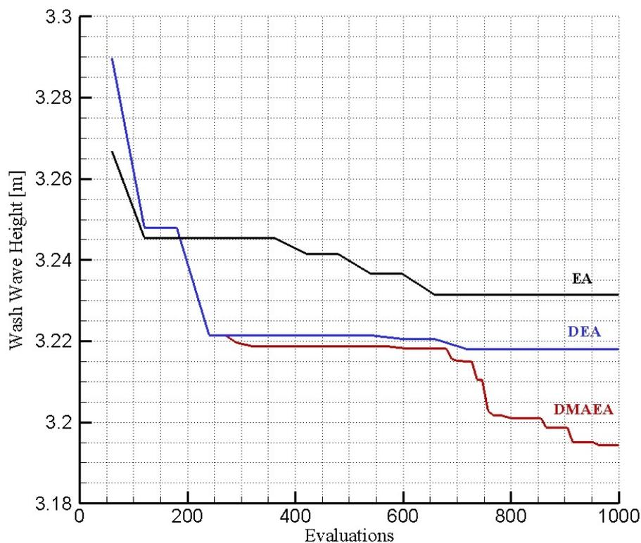
Figure 3: Fast displacement hull form design. Comparison of the EA, DEA and DMAEA for the single objective optimization (SOO) problem.
