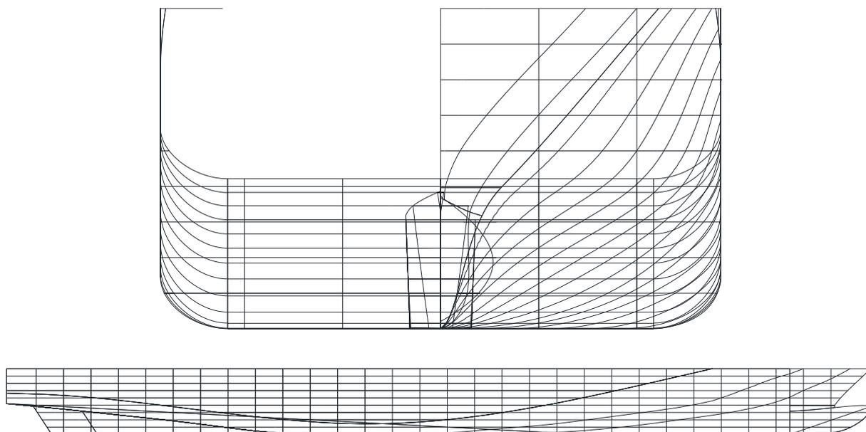
Figure 5: Body Plan and Profile of the optimized C3-opt1 fast displacement hull form (17 parameters, DMAEA).
