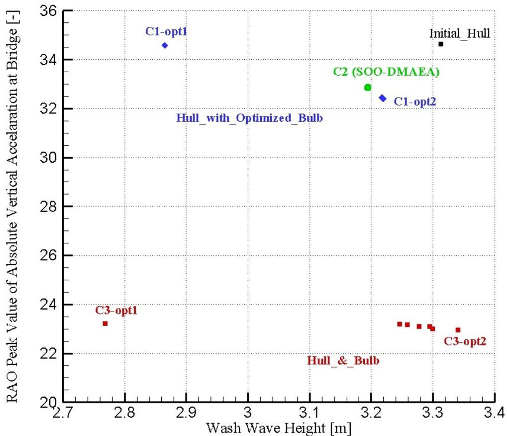
Figure 4: Fast displacement hull form design. On this figure the SOO results for the bulb only and the hull & bulb are presented. The respective MDO Pareto front is derived via DMAEA.
