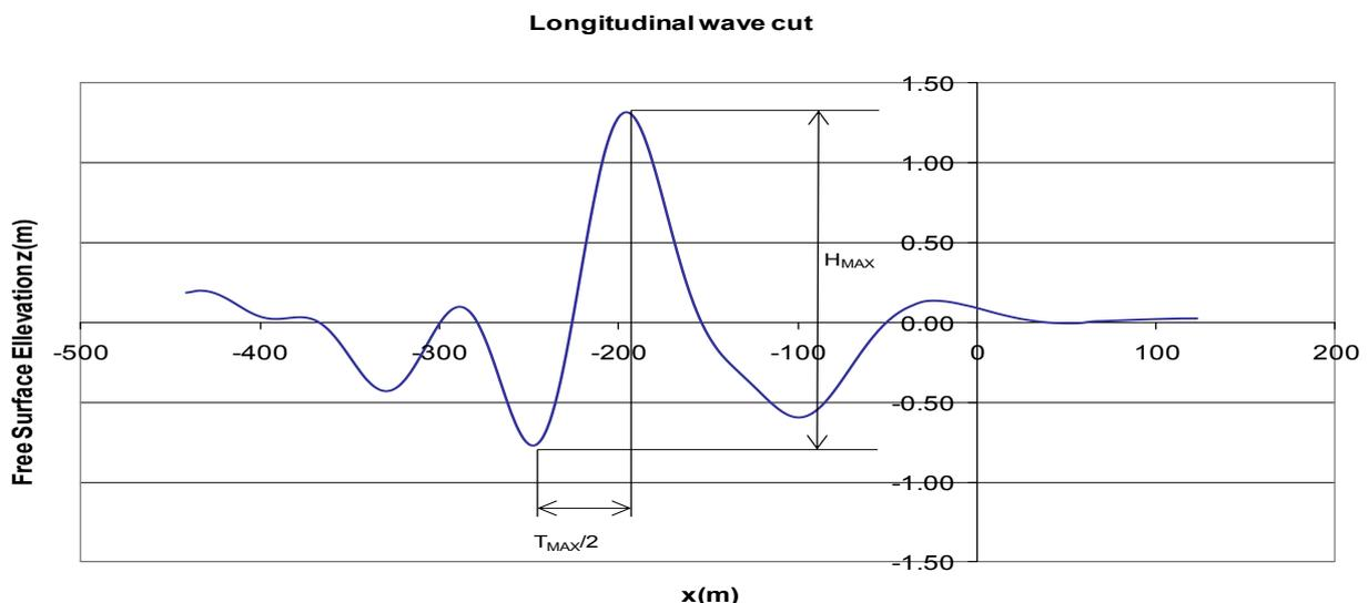
Figure 1: Longitudinal wave cut for the definition of the maximum wave height of wave wash.
