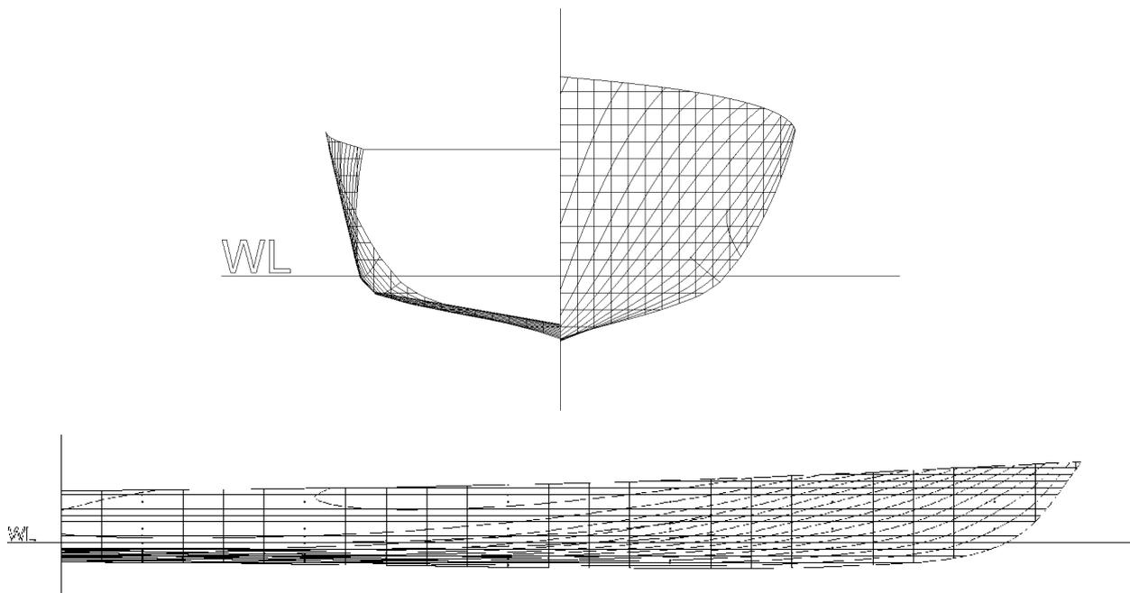
Figure 6: Body Plan and Profile of the parent of the double-chine hull form
