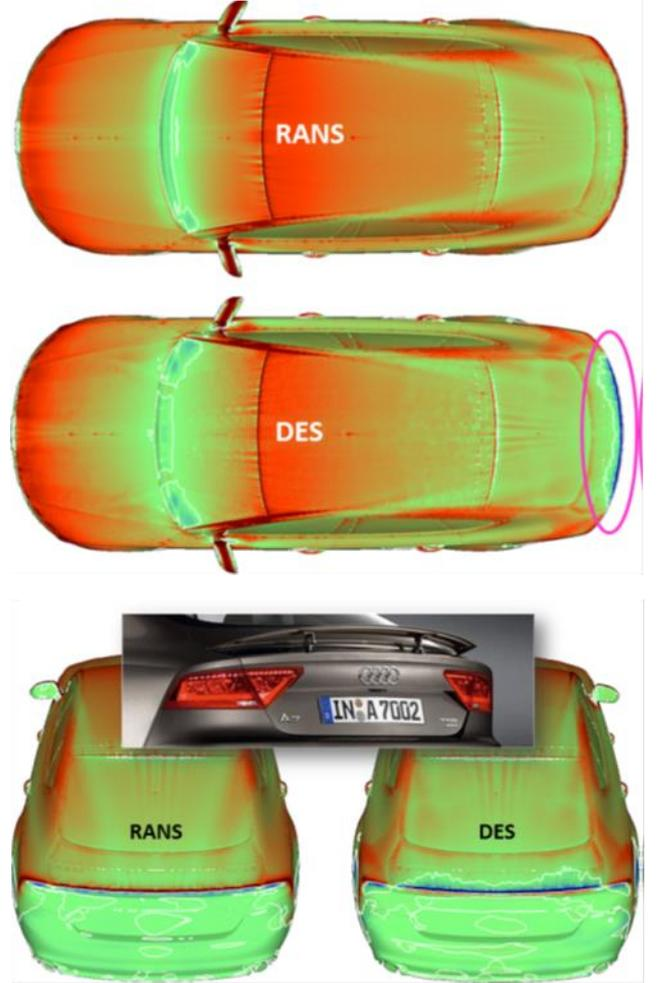
Fig. 3: RANS vs. approximate DES sensitivities for Audi A7. The actual shape of the active spoiler in the current Audi A7 is shown in the bottom of the image.
