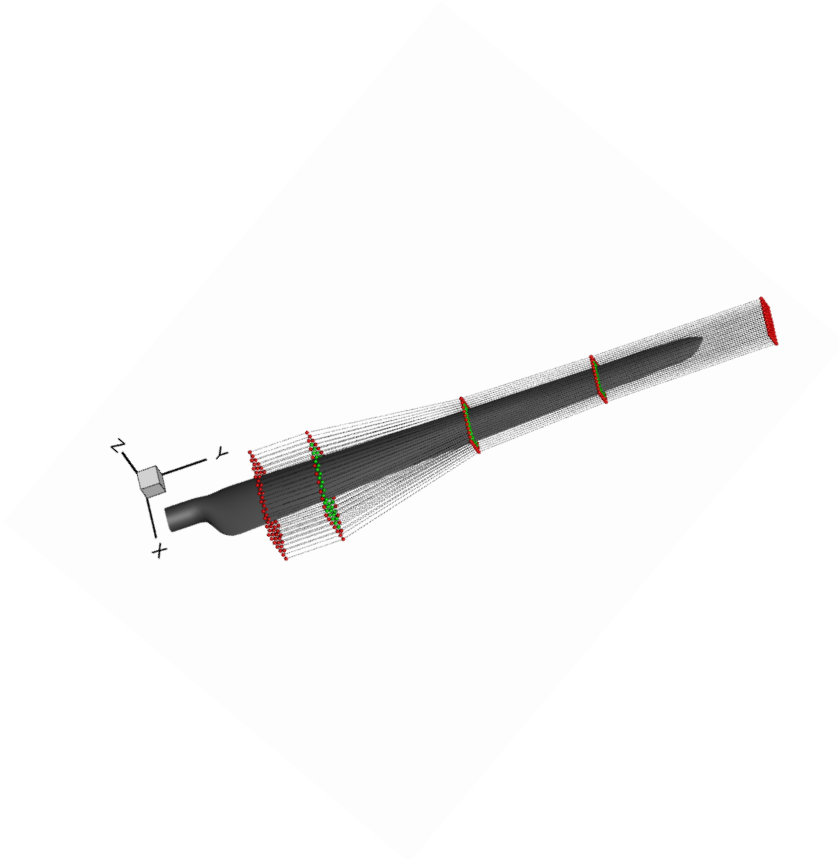
Fig. 3 Parameterization of the HAWT blade.
