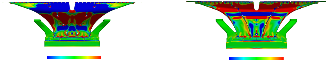
Figure 8: Sensitivity map indicating the change in the objective function F caused by the normal displacement of the boundary faces. Blue-colored areas should be pulled outwards while red areas should be pushed inwards so as to decrease the value of F .
