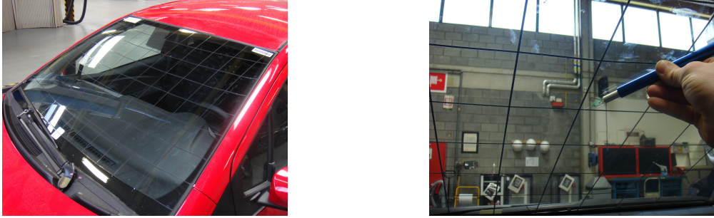
Figure 4: Set-up of the velocity pattern measurement. On the left, the 100mm-spaced grid is shown while, on the right, the use of the hot-wire anemometer on one of the grid points is demonstrated.
