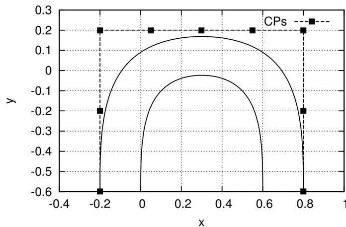
Figure 1: 2D U-bend duct optimization: duct shape and the Bézier–Bernstein control points parameterizing it. Only the  $y$  coordinates of the top 5 control points (CP) are allowed to vary during the optimization.
