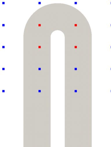
Figure 6: 3D U-bend optimization: Part of the duct shape along with one of two iso- $z$  control point planes. Red control points are allowed to vary while blue ones are kept fixed during the optimization.
