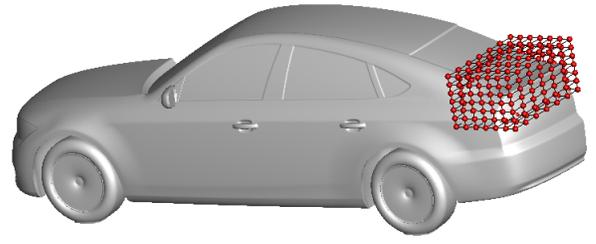
Fig. 9. Shape Optimization of the fastback DrivAer Car: NURBS morphing box. Only the rear part of the car which is encapsulated into the morphing box is allowed to change during the optimization loop.
