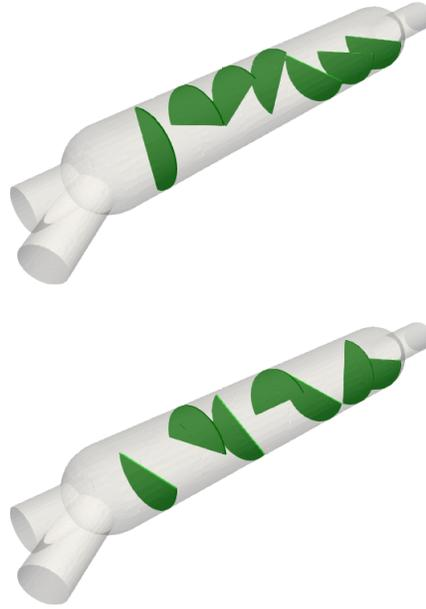
**Figure 13:** *Positional Angle Optimization. Final positions of the baffles for the two extreme Pareto solutions. Top: positions when optimizing only for  $F_P$ ; bottom: positions when optimizing only for  $F_U$ .*
