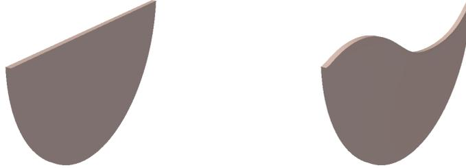
**Figure 5:** *In-plane optimization. Example of the modification of the profile of an arbitrarily selected baffle. Initial flat-lined profile (left) and the outcome of the optimization (right).*
